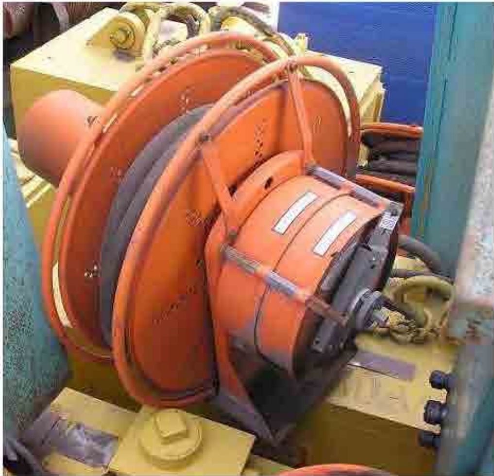
6. MMD cable reel with cable
