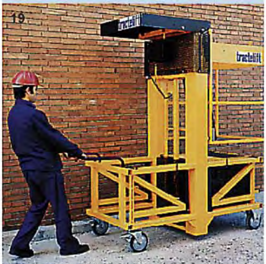
TRACTELIFT mobile work platform • max. height of the floor panel 7.3 m to 10.3 m (according to the model) • maximum load: 225 kg • power supply by rechargeable battery • standard model with swivel wheels • towable model (optional)
