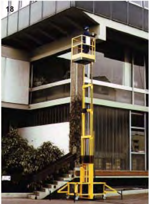
TRACTELIFT mobile work platform • max. height of the floor panel 7.3 m to 10.3 m (according to the model) • maximum load: 225 kg • power supply by rechargeable battery • standard model with swivel wheels • towable model (optional)
