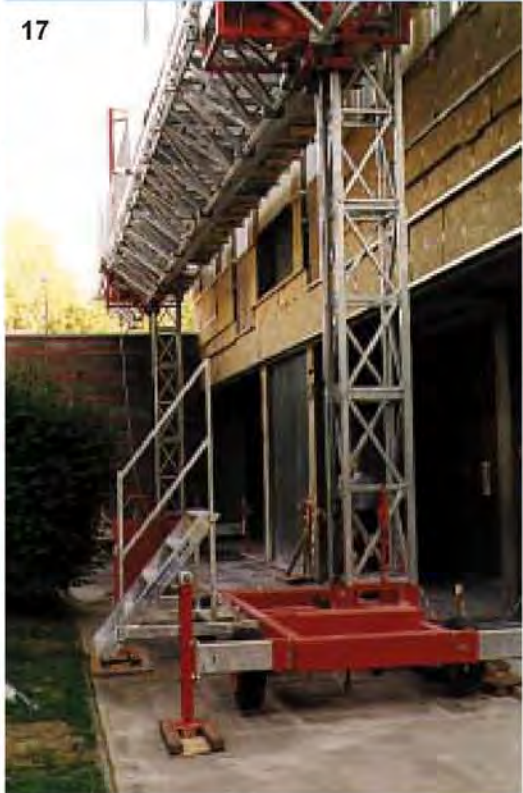
ELECTROSCAF 3000 working platform with a single or double mast • maximum height: 150 m • max. load (evenly spread): 1200 or 3000 kg • maximum length of platform: 10 or 24 m
