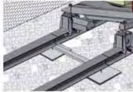
Rail track placed on concrete or steel plate
