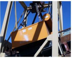
The Series 7000 magnets can be easily adapted for special applications like this foundry sand reclaiming line. This unit is designed to applications having larger than normal amounts of tramp iron and where the tramp iron is hot, sharp, or large in size. These foundry magnets are equipped with a heavy duty high-temperature belt and oversized drive components as well as heavier frames, bearings and pulley shafts.
