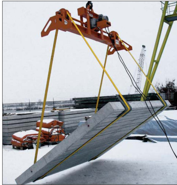
422 572: WTVE 4.5/2 , carrying capacity 4.5 t, manually adjustable working width of 1.0 to 2.0 m 422572: WTVE4.5/2, 承載能力4.5T, 手動調節工作寬度1至2m
