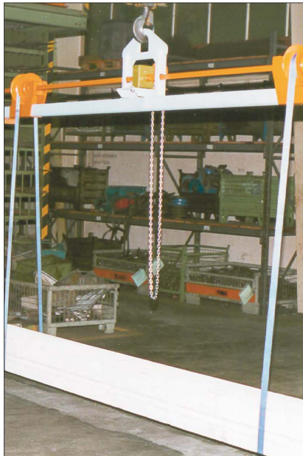
WTV 0.8-0.3 : manual load rotating beam with low construction height, carrying capacity 0.8 t WTV0.8-0.3: 手動荷重旋轉吊樑, 低搭建高度, 承載能力0.8T
