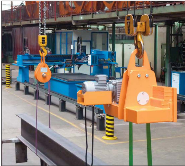
422 584 / 422 585: load rotating device WTE 2.0 complete with load rotating drum WT 1.0 , total carrying capacity 3 t 422422/584585: 荷重旋轉裝置WTE2.0完整的設備附有荷重旋轉滾筒WT1.0總承載能力3T
