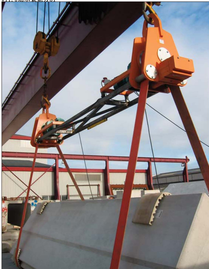
422 556: Two load rotating devices WG 12.5 with distance frame, total carrying capacity 25 t 422556: 兩個荷重旋轉裝置WG12.5附有距離的框架, 總承載能力25T
