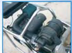
RT66/RT74 Honda GX120 with Dual Air filter as option
