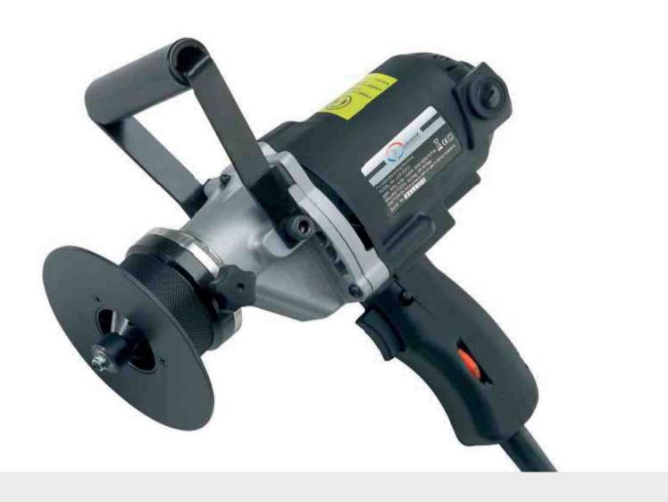
The LKF.450/2 machine is perfectly suited for making welding angles, to countersink drilled holes and to deburr material. Thanks to the variable adjustable speed, this machine is can also be used for strong steel next to mild steel. The LKF.450/2 is powered by a strong 1100W motor, which is equipped with a 'soft-start' feature.
