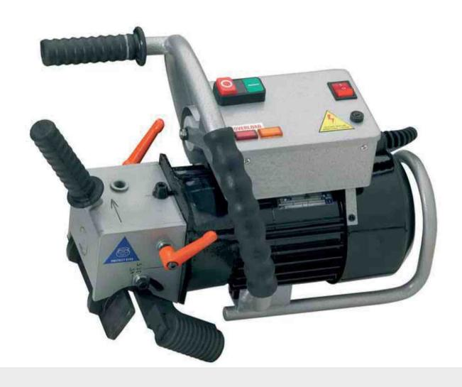
The LKF.200 is designed to bevel angles between 30 and 60 degree steel edges prior to welding. It is reliable and simple to use. The LKF.200 machine can be used for beveling straight steel sheets and pipes. It allows you to bevel steel edges between 15 and 60 degrees. Maximum face of bevel is 20 mm (3/4"). When equipped with special attachment it can also work on pipes above 150 mm (6") diameter.
