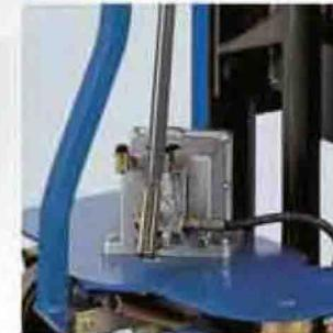
Manual traction and elevation lift trucks: the lift of the forks takes place thanks to a double-acting pump; the descent takes place through a handwheel situated on the machine body.
