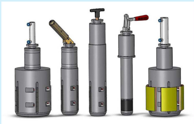
Left to right: 6" mandrel with pneumatic retract, 3" toggle retract, 3" "T" handle retract, 50 mm urethane mandrel with locking toggle handle and 6" leaf-type mandrel with pneumatic expand and retract. 從左到右依次為：6"附有氣動退回軸心，3"切換退回，3"“T”把手退回50mm聚氨酯芯軸與鎖定切換處理和6"葉型心軸附有氣動膨脹和退回
