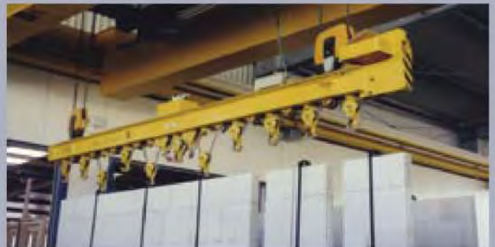
Balance crosshead with integrated electro chain gear to shorten the suspension chain
