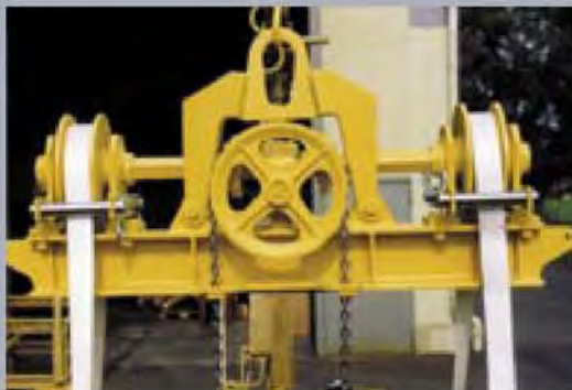
Turning crosshead with worm gear pair drive
