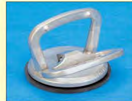
Model 600.0 Cast aluminum body, one-hand operation. 4-3/4" diameter cup. Horizontal use. Carrying capacity: 33 lb (15 kg)
