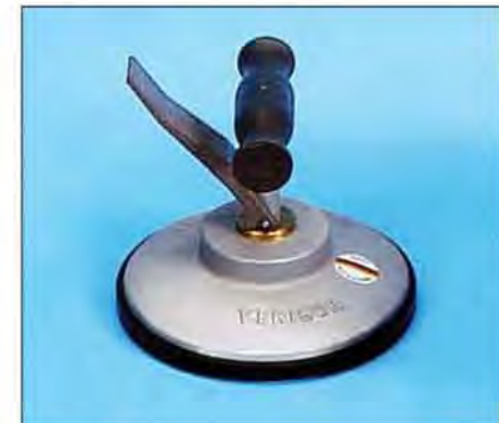
Model 608.0 Lever creates vacuum in down position. For floor tiles, artificial slate, ceramic, marble, granite, etc. 7-3/32" diameter. Horizontal use only. Carrying capacity: 66 lb (30 kg).
