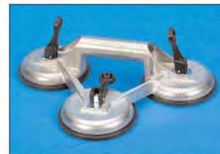
Model 603.0 Cast aluminum body with three cups. Useful for large-sized sheets of material. 4-3/4" dia. cups. Carrying capacity: 110 lb (50 kg)
