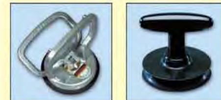
Model 600.5 Cast aluminum body, one-hand operation. 3-1/2" diameter cup. Horizontal use. Carrying capacity: 22 lb (10 kg). Model 609.2 has a 3-1/8" dia. body. Rubber, with metal T-grip.
