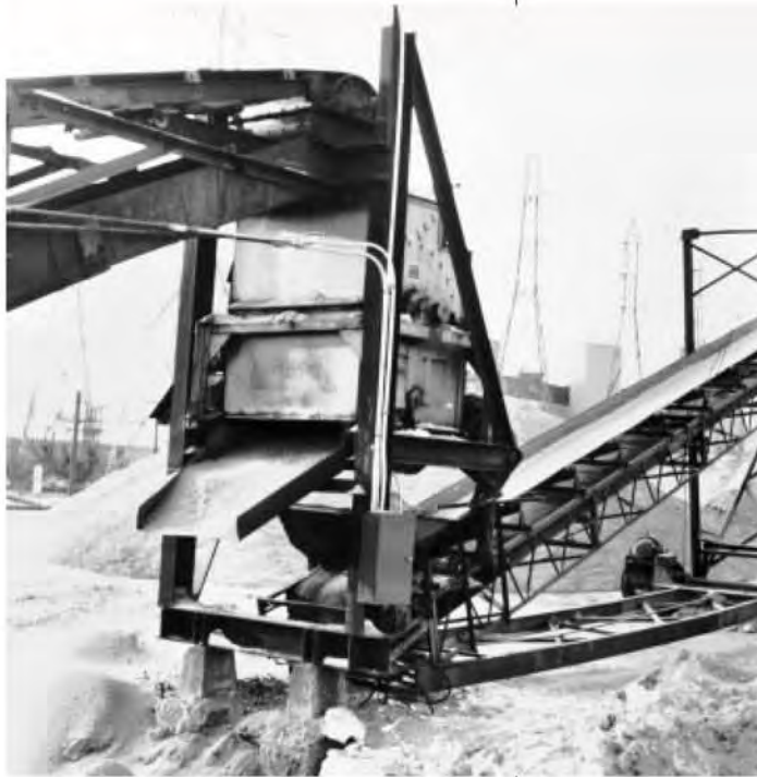
Single Stage DF Separator removing ferrous contamination from slag for use in cement block manufacture.
