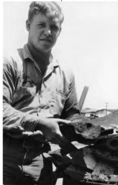
Figure 3. Large Pieces of Tramp Iron Automatically Removed from Processing Line
