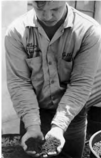
Figure 2. Fine Iron Contaminants Removed from Three-Inch Burden Depth
