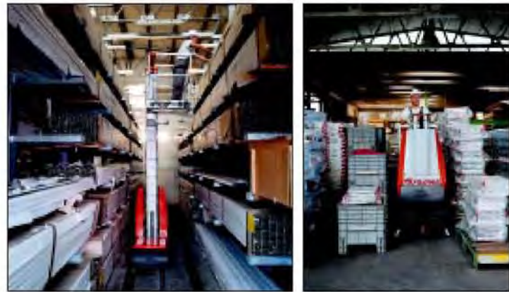
Articulated platform: One man platform providing overhang access over 360°.
