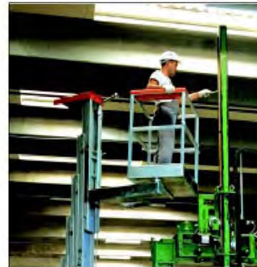
Rotating platform, allows work closer to the object.
